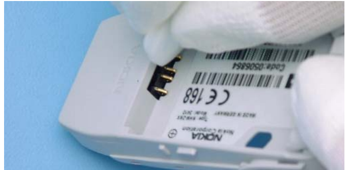
There are different ways to remove the Battery Connector. One way is, to press it from the backside of the D-Cover. The other way is to take it with fingers from the front side of the D-Cover.
