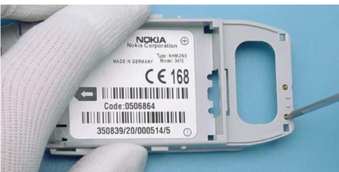
You need some power to press the Antenna Pogo Pins from the D-Cover.
